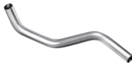
Stainless steel pipe 48,3 x 2 mm, bent on TUBOBEND 50
