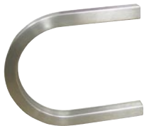
Square tube 20 x 20 x 2 mm, bent on TUBOBEND 50
