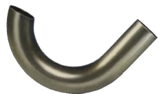
CuNiFe pipe 42 x 2 mm, bent on TUBOTRON 50
